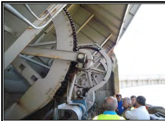
Figure 49 – Trunnion Rack, Spur Gear and Earle Gear Reducer
